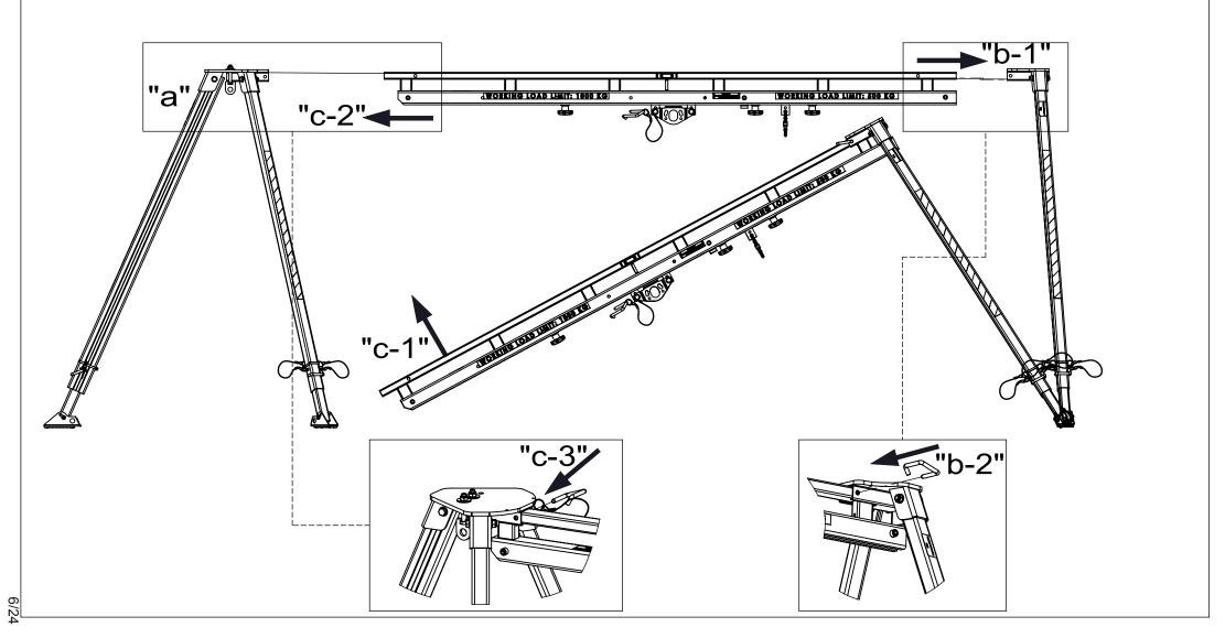
LEVELING SPIDER BEAM / LOCKING TROLLEYS POSITION WITH T-LOCKS Always ensure that the beam is true and level using mounted spirit level before use. Improper leveling may result in self displacement the load being lifted along the beam which can cause injury to the operator.
