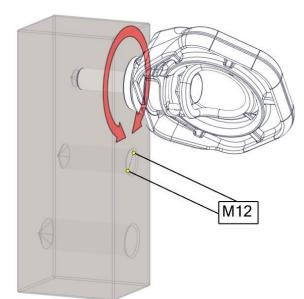
Figure 4. Installation of anchor point
