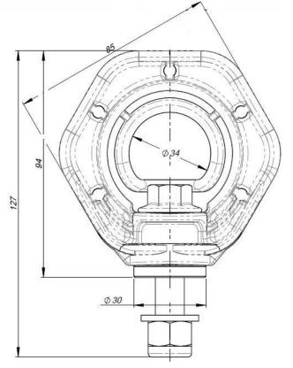
Figure 2. Overall dimensions AT185
