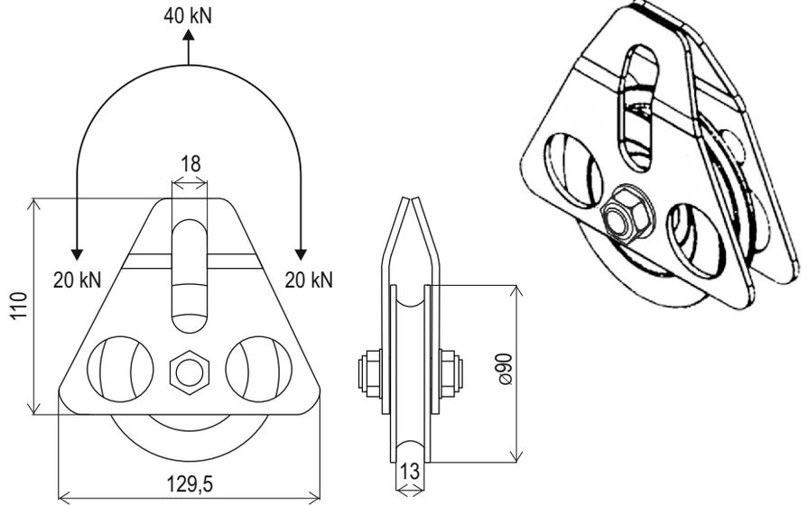
**USE OF PULLEY PL101 FOR LIFTING OF LOADS**
