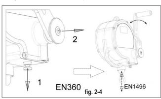
The switching from EN360 to EN1496 function may be done especially when the CRW200 have arrested a fall and there is neccesity to rescue of the user. In order to change the EN1496 function to EN360 pull out the locking pin "1" and next push in the crank axle "2" inwards (fig. 2-5). Than the device will act as a retractable fall arrester.
